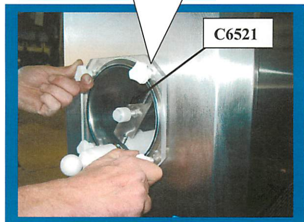
Installing small Faceplate onto front of Machine.
