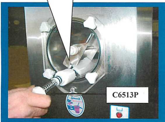
Installing Plunger Assembly into Faucet body
