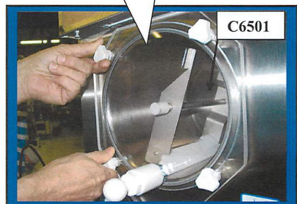
Installing Faceplate onto front of Machine.
