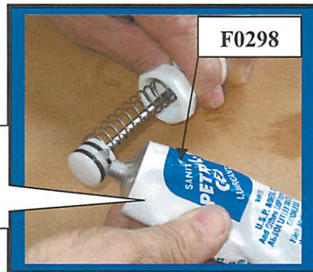
Lubricating o-rings with Petro-Gel
