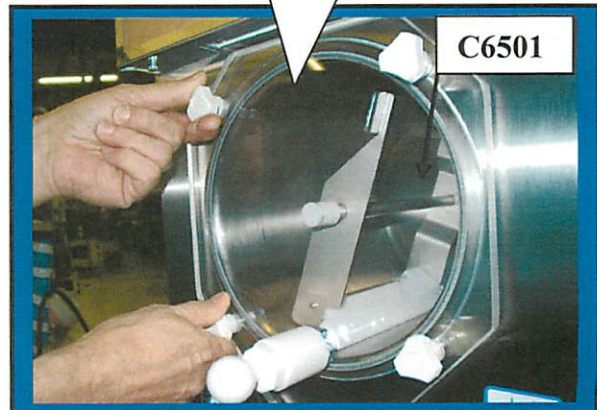
Installing large Faceplate onto front of Machine.
