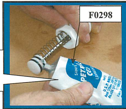
Lubricating o-rings with Petro-Gel
