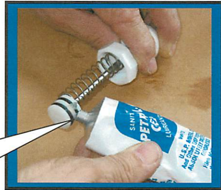
Installing o-rings onto plunger F 0491
