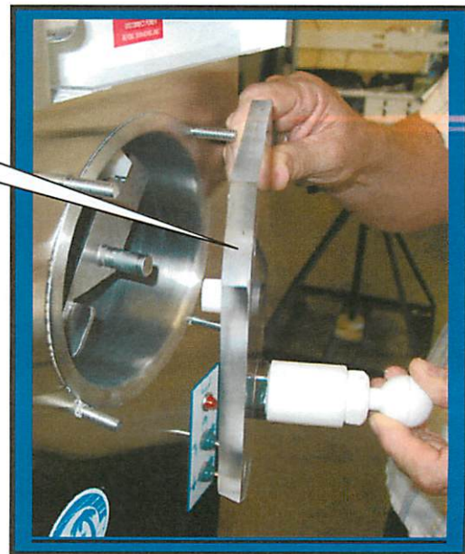
Installing faceplate C6521 onto front of Machine.
