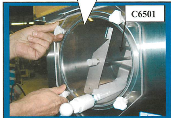
Installing large Faceplate onto front of Machine.
