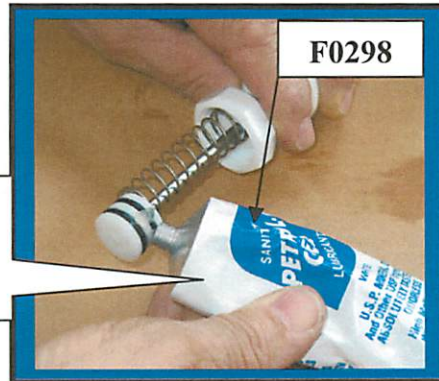
Lubricating o-rings with Petro-Gel
