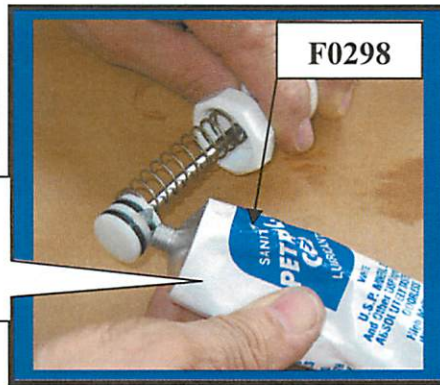
Lubricating o-rings with Petro-Gel
