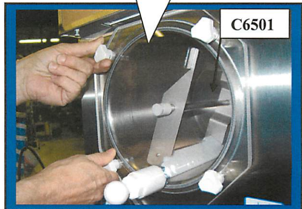
Installing large Faceplate onto front of Machine.
