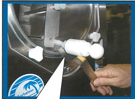
Align Faucet Assembly opening to bottom of faceplate then tighten nut
