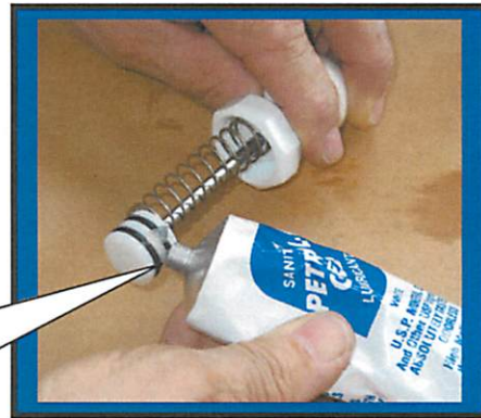
Lubricating o-rings with Petro-Gel F0298
