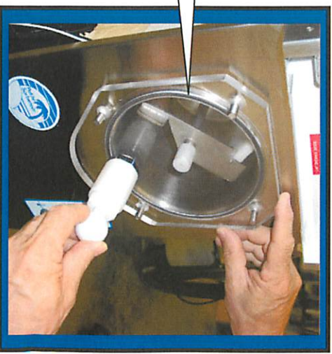
Step 7: Install beater bar C6519 into cylinder.
