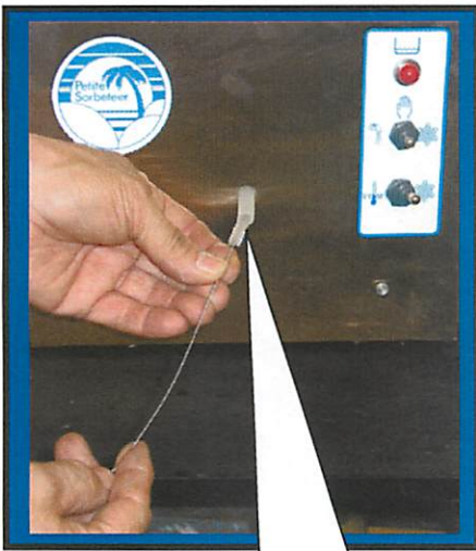
Insert long brush F6526 into drip tube
