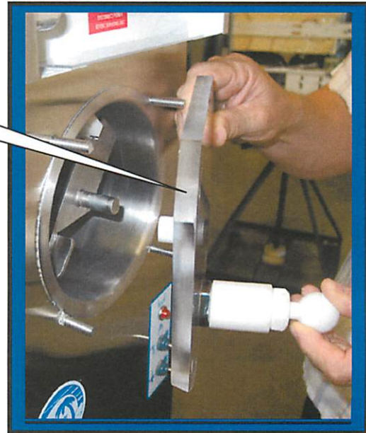
Installing faceplate C6521 onto front of Machine.
