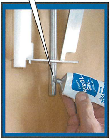
Step 4: Apply a small dab of Petro-Gel F0298
