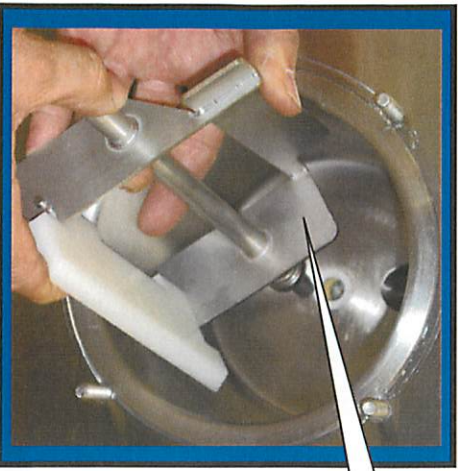
Step 7: Install beater bar C6519 into cylinder.
