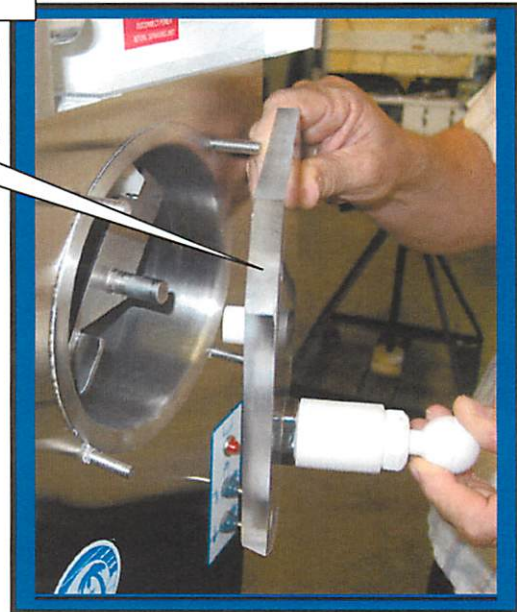
Install faceplate C6521 onto front of Machine.
