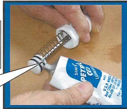
Install o-rings F0491 onto plunger
