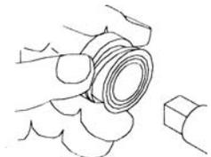
**Figure U** Re-assemble rotary half of seal as shown
