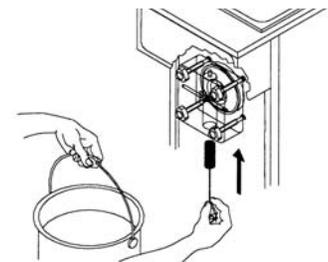
**Figure T** Clean Valve Body
