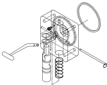
**Figure M** Disassemble Dispensing Valve
