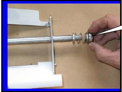
Step 5: Install spring seal F0355
