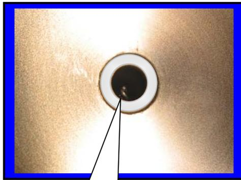
Push brush all the way in until it can be seen in the middle of the ceramic ring
