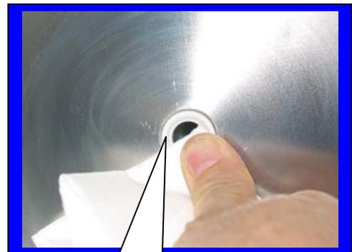
Clean ceramic ring with warm, wet rag. Remove any dried product from center of ceramic ring.
