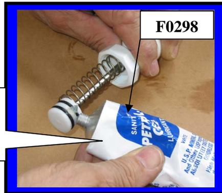
Installing **Plunger Assembly** into Faucet body
